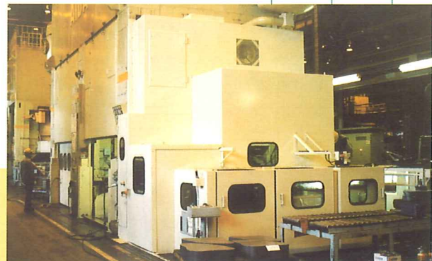
Sound-proof Enclosure for 2500ton Transfer Press Machine
